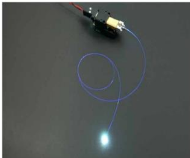
Figure 7. Nichia's First White Laser Light Source [13]
